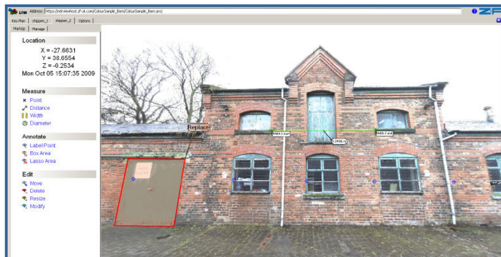
LFM NetView BubbleView interface. Blue dots indicates adjacent scan positions hidden from view.
